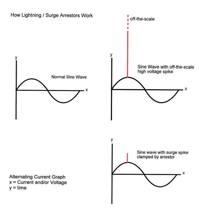
Clamping voltage varies by rate of surge rise, wave-shape, and current magnitude.
